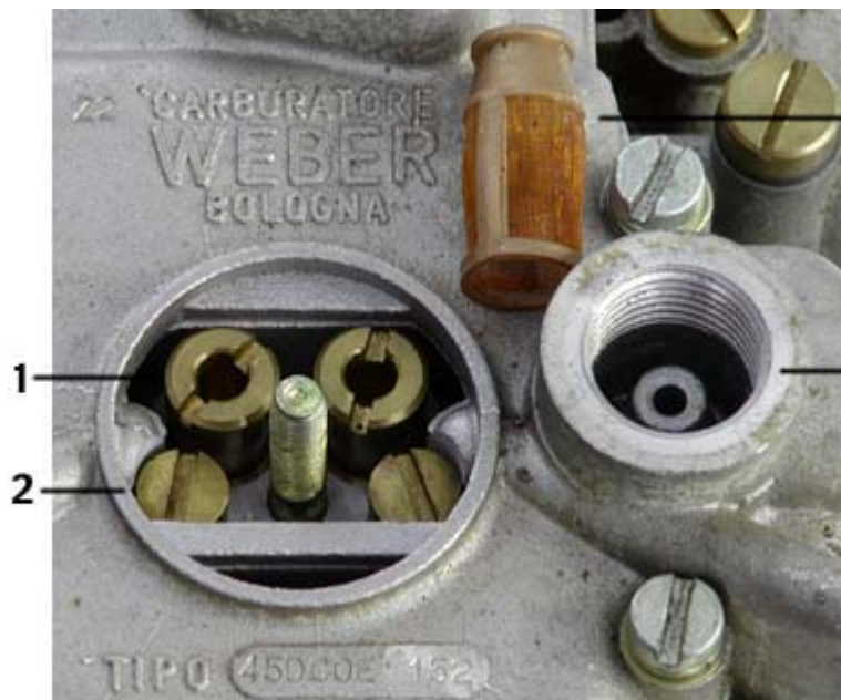
3 Top of a DCOE with centre cover and fuel filter cover removed
